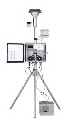
The Exactus BAM is a portable, real-time beta gauge which is comparable to U.S. EPA methods for PM<sub>10</sub> particulate measurements.
